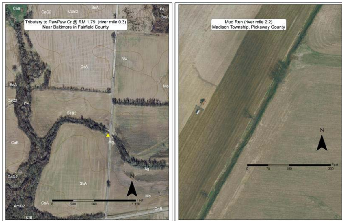
Figure 8.8 Aerial photos showing sources of stress to a tributary to Pawpaw Creek (left) in Fairfield County and Mud Run (right) in Pickaway County. The left photo shows the partially impaired site (yellow triangle) as well as a clear illustration of the level of intensity of subsurface drainage use (evidenced by the drier, lighter colored soil above the drainage tiles). Soil map units are also included to illustrate the dominance of loamy soils in the area which, when drained, leads to higher peak discharge. The right photo illustrates drainage ditch maintenance approximately 0.6 miles upstream of a biological survey site that failed to meet any of the biocriteria.
