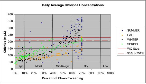
Figure 3: Concentration-Flow Duration Plot for Station 193-NTC-01
