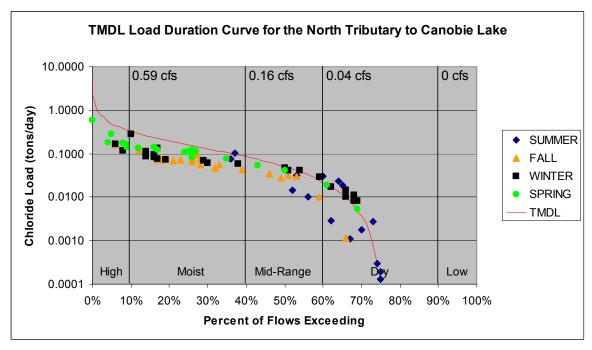
Figure 5: TMDL Load Duration Curve at Station I93-NTC-01
