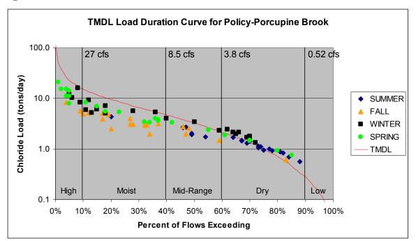
Figure 5: TMDL Load Duration Curve at Station I93-POL-01V
